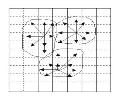
$$f(x) = \frac{CoverRate(x)^{\alpha}}{NumberTransmittersUsed(x)}$$
