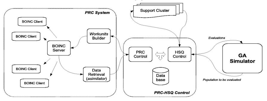
Schema similar to the previous one, but it includes a modified PRC control module (PRC-HSQ control) and a centralized and defined characteristic. As previously stated, the function of this module is to decide if the work must be assigned to the support cluster instead of submitting it to the BOINC based PRC system.
