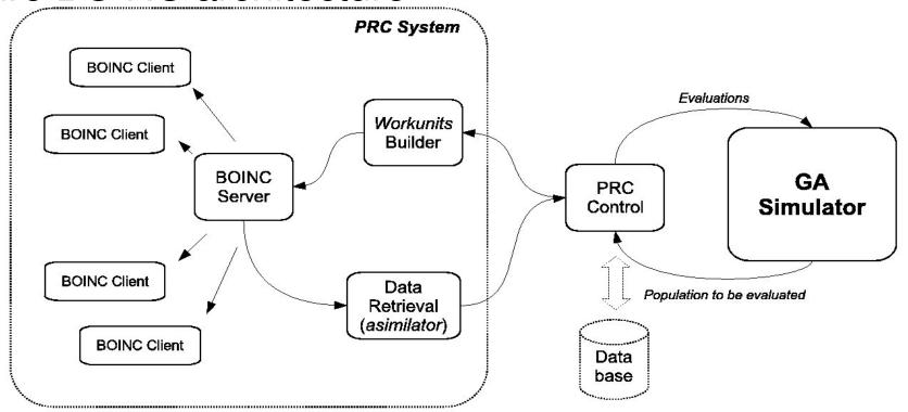
Modification of the GA simulation library for executing the evaluation function corresponding to each individual for the active generation
